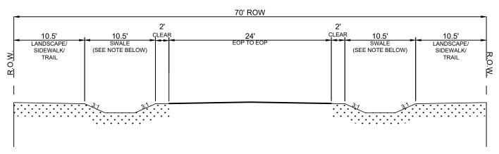
NOTE: THE CITY ENGINEER MAY APPROVE A REDUCED ROADSIDE SWALE WIDTH IF IT CAN BE DEMONSTRATED THAT THE REDUCED WIDTH WILL FULLY CONVEY DESIGN STORM EVENTS (IN ACCORDANCE WITH COA DCM)
